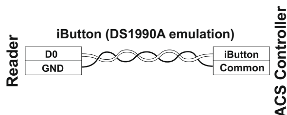
Fig. 5. Connecting the reader to ACS controller.
