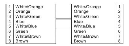
**ETHERNET** RJ45 connector to join LANs. Requires a standard straight Ethernet patch cable.
