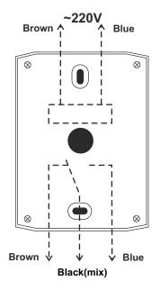
Power Relay Control Cable (3 wires)
