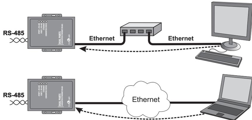
This mode is convenient when the converter IP address is known or the network settings and structure allow the software to detect it.
