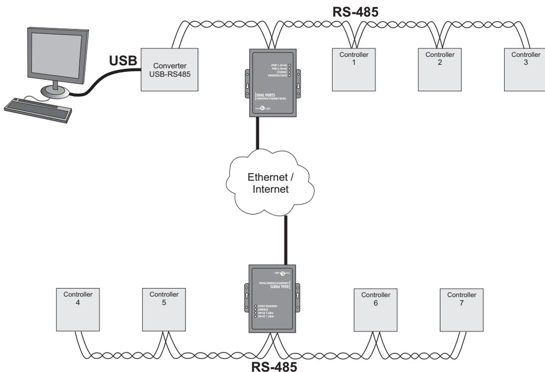
Ethernet bridge mode configuration example.
