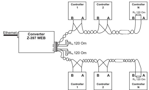
Example connection layout for converter plugged into the middle of RS-485 chain. No terminating resistive load required to connect to Z-397 WEB.
