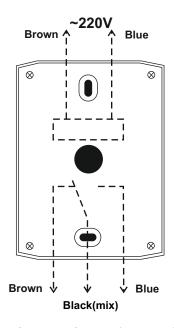
Power Relay Control Cable (3 wires)
